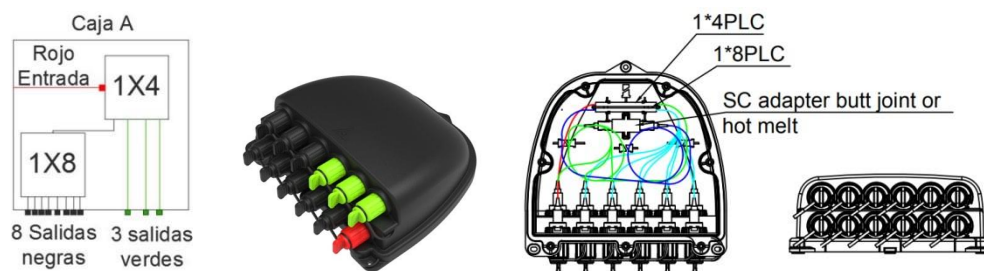
MINIBOX68-12-S4S8 (1 * 4 PLC + 1 * 8 PLC Splitter Cable Ways)
