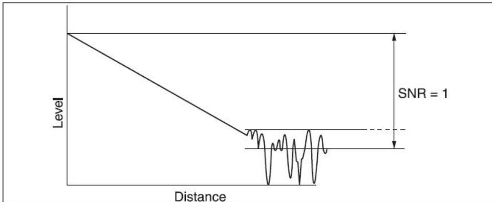
④ Dead zone is measured with pulse width of 3ns and return loss under -55dB.
