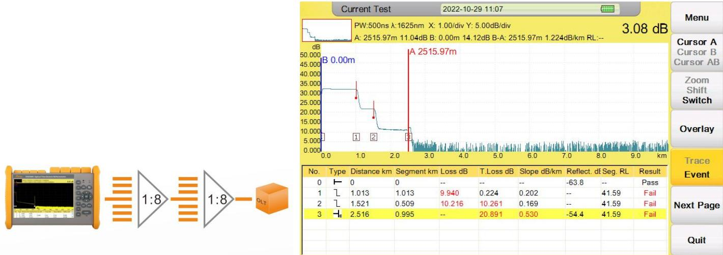
In particular, with FLM mode, users can automatically test without complicated settings to obtain the most accurate and intuitively test results. In addition, FLM provides the Pass/Fail function of the PON network, which can intuitively display the failure event in PON network
